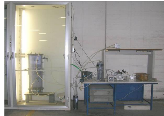
Anaerobic Membrane Bioreactor (Progetto Aquafit 4use)
